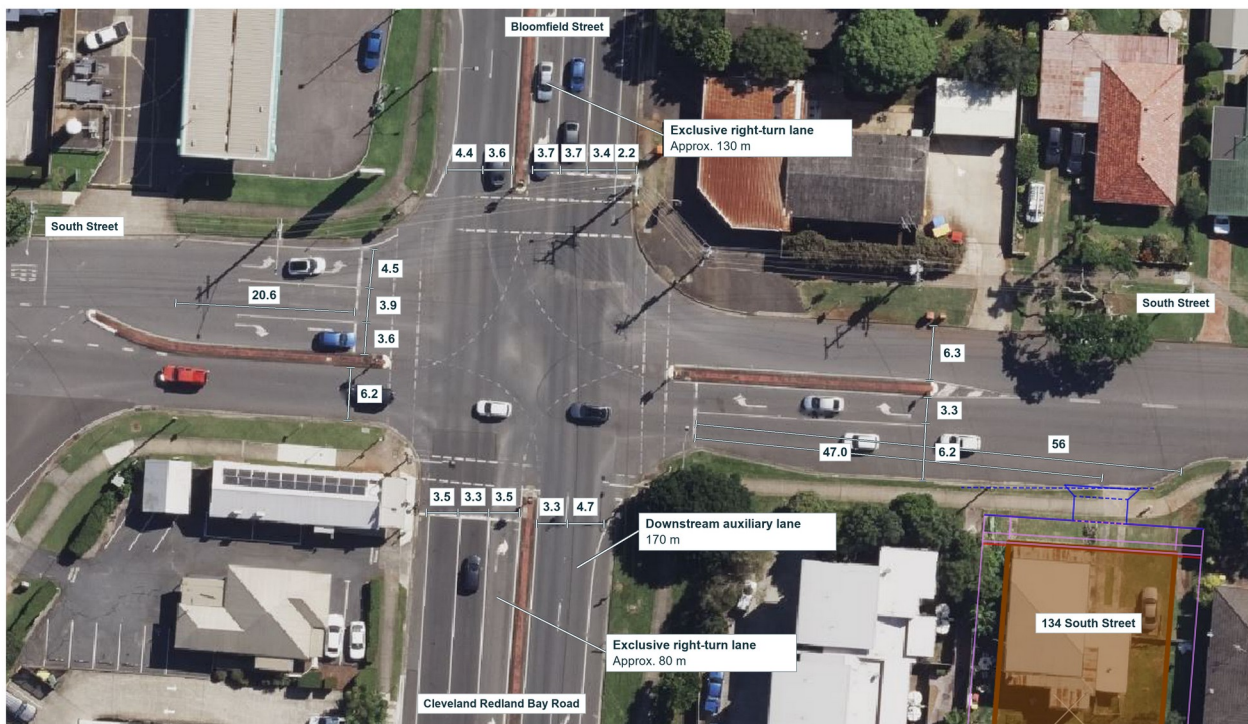
Figure 2: Intersection geometry, South Street / Bloomfield Street / Cleveland Redland Bay Road. Lane widths and turn-bay lengths in metres as annotated; approximate lengths as shown, not to scale.
