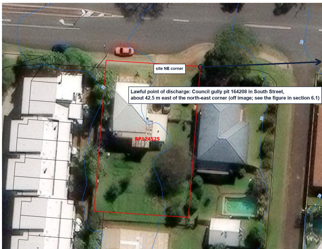
Figure 2: Site (Lot 1 on RP124525) with the direction to the lawful point of discharge, Council gully pit 164208 in South Street (owner-supplied aerial, annotated)
